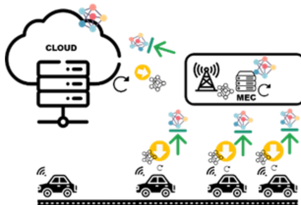
Figure 10: Federated Machine Learning for automotive verticals involving model training, aggregation, and transfer (using Edge server and OBUs)
